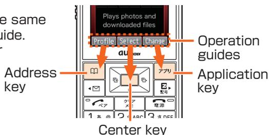
Various functions are assigned to the 3 keys depending on the screen in operation.
